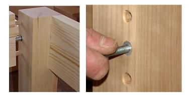
4. Attach the side rails to the footboard panel (see images on the previous page), then loosely secure using the half-moon washer and the nut with the spanner provided (see image below). In the same way attach the side rails to the headboard to create a full bed frame.
