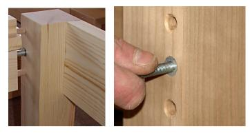
3. Attach the side rails to the footboard legs (see images on the previous page), then loosely secure using the half-moon washer and the nut with the spanner provided (see image below). In the same way attach the side rails to the headboard to create a full bed frame.
