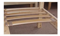
You can make the 'feel' of the slat base firmer by moving the sliders out to the edges (as shown above). For a softer/more flexible feel move the sliders towards the centre of the slats (towards the top of the curve of the slats).
