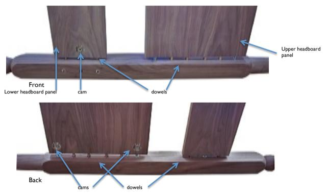
5. Use the hexagon key to tighten all the cams:
