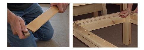
Counting from the headboard end – the fourth slat will be a double slat (made up of an upper standard slat to which is attached a lower second slat via a plastic slider) – see image below. Slats 4-9 will be double slats, the others are standard single slats (see image below).
