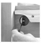
2. Next build the headboard: take one of the two posts that have the large mortise slots in them (see the first image above) and insert the timber edge of the upholstered panel within the slot. Attach the lower headboard rail to the post using the half-moon washer supplied. Do the same to the other side using the remaining post with the mortise slot. N.B pay attention to the numbers and ensure they correspond.
