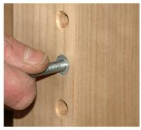
3. Attach the side rails to the footboard panel, then loosely secure using the half-moon washer and the nut, with the spanner provided (see image below). In the same way attach the side rails to the headboard to create a full bed frame.
